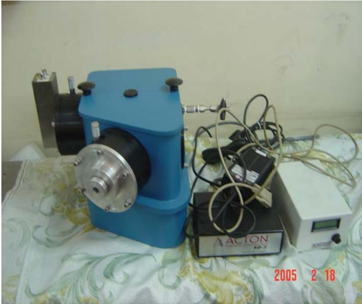
8. Vibration Shaker used for structural health monitoring and structural vibration control. A wide band random vibration with three-sigma excitation of 10g is introduced on to real aircraft fin tip and it has been demonstrated that 80% reduction in vibration level is achieved using robust control implemented using Indigenous DSP based system and high voltage amplifier. This results compares favorably with that achieved recently for F-18 Aircraft in USA.
