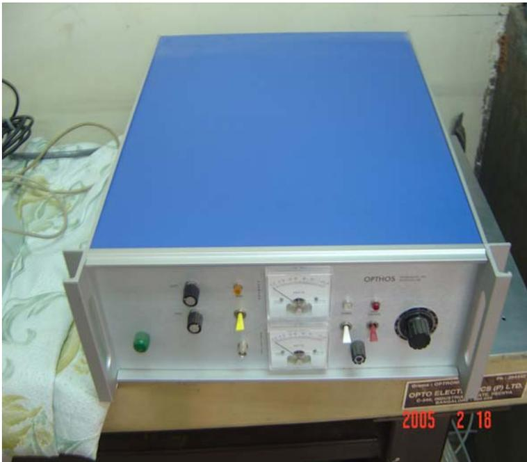
7. Vacuum Monochromator used for identifying the transient species in high temperature reactions using atomic resonance absorption spectroscopy.
