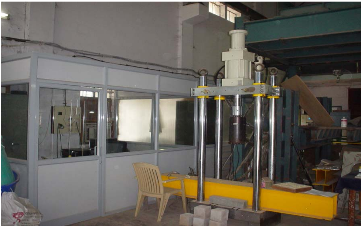
Photograph 7: View of the Upgraded 500 kN Servo Hydraulic Actuating Test Facility. Also Seen Is the Control Room Housing the Computer Based Controller and the Hydraulic Power Pack
