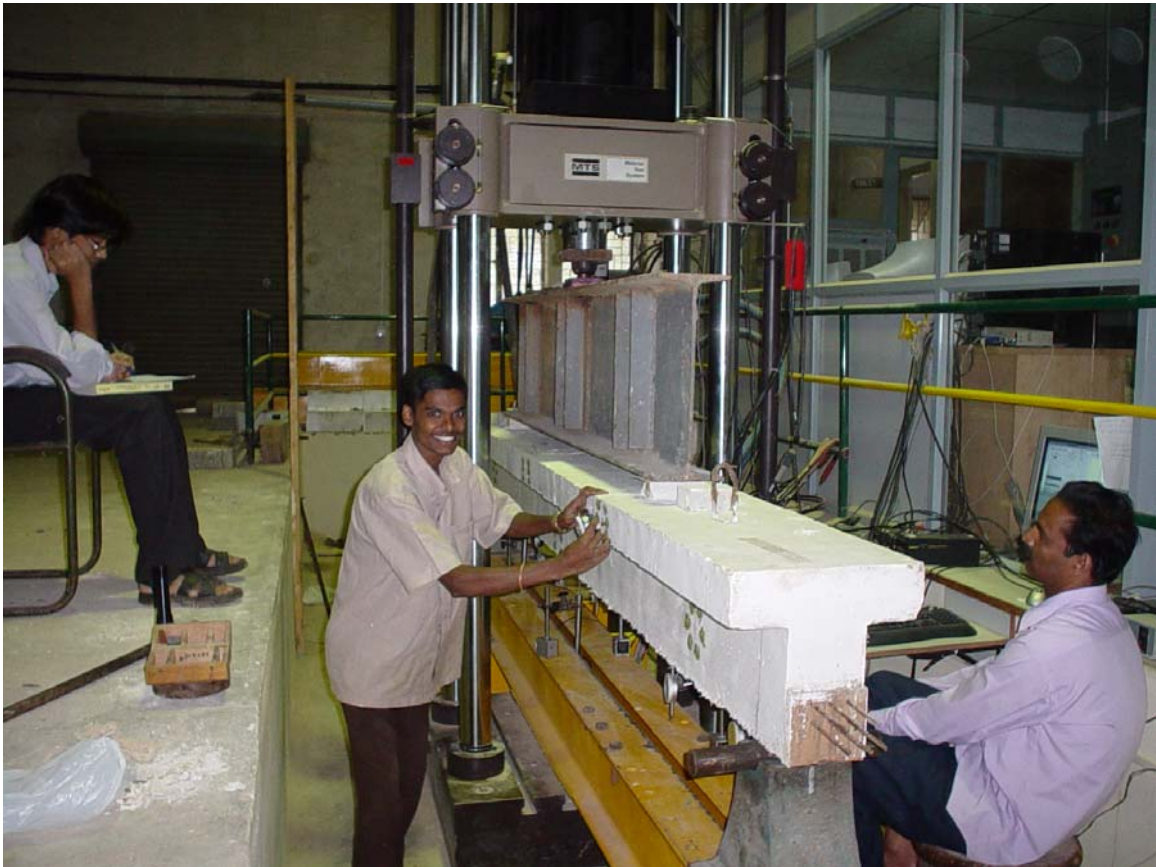
Photograph 1: Prestressed Concrete T-Girder Specimen Being Tested in the MTS 1200kN Material Testing Facility. Also in View is the Strong Floor Created to House the Load-Frame
