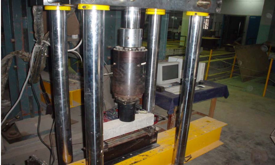
Photograph 8: View of the Upgraded 500 kN Servo Hydraulic Actuating Test Facility. Also Seen is the Computer Based 8-Channel Acoustic Emission Facility
