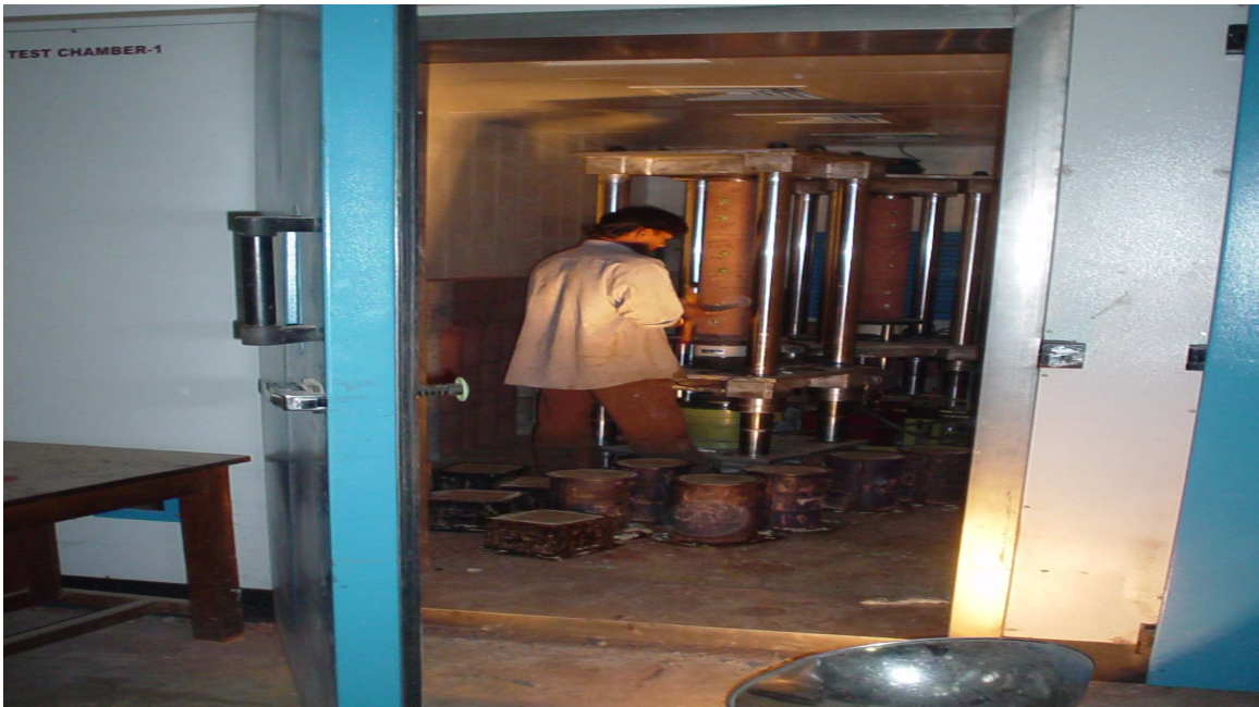
Photograph 4: View of the Open Walk-in Humidity (40% -98% Relative Humidity) and Temperature (20-50 degree Celsius) Controlled Room Housing 1000kN Self-Reacting Frames for Studies on Creep in Concrete
