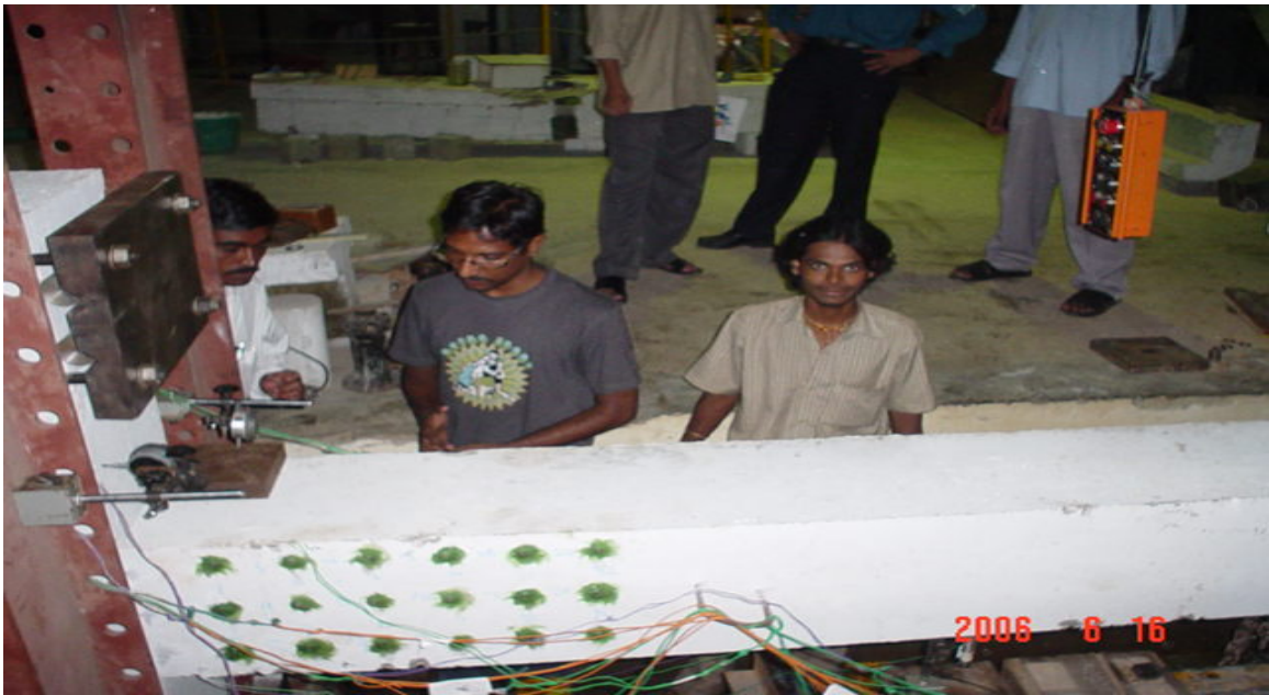
Photograph 3: Exterior Reinforced Concrete Beam- Column Joint Being Instrumented Prior To Testing In MTS Material Testing Facility
