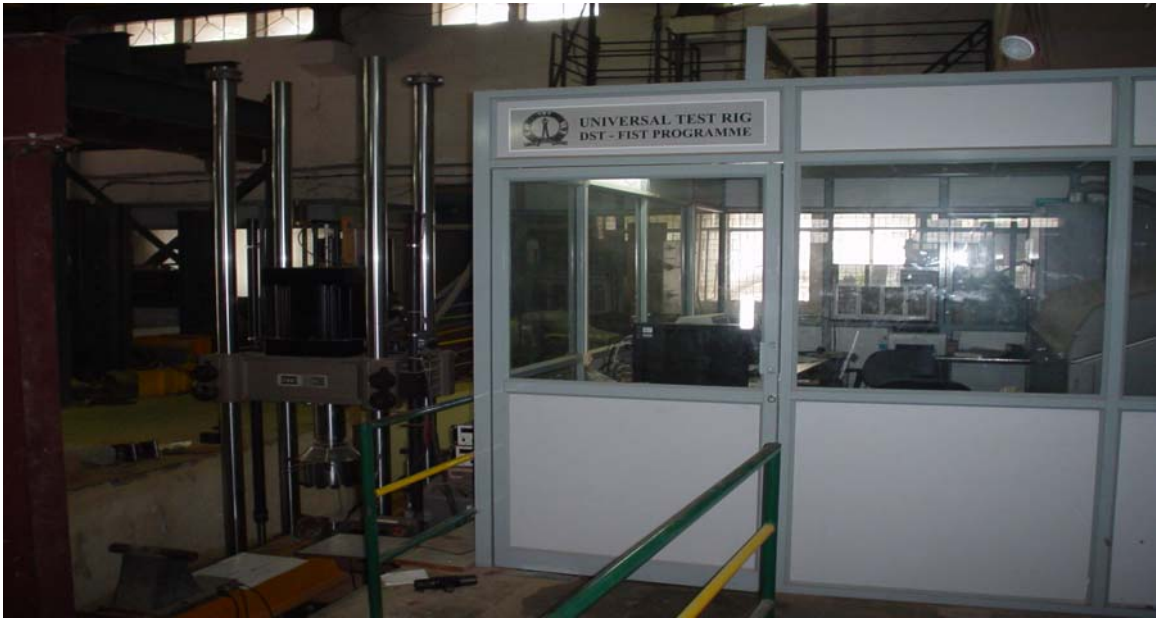
Photograph 2: View of the 1200kN MTS Material Testing Facility-Load-Frame, Actuator, Control Cabin Housing the Computer Based Controller and Hydraulic Power Pack
